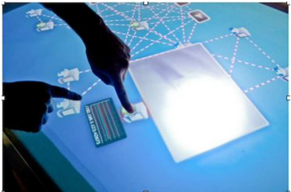
Figure 3. By touching a producer node you will see a preview of the video stream. The small graph underneath shows real-time CPU load measurements.
