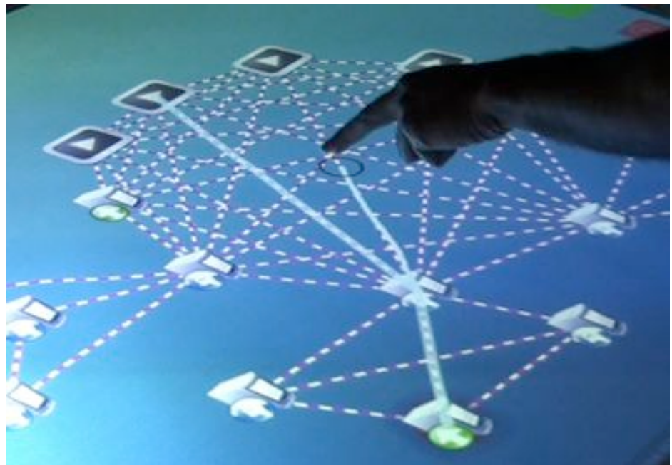
Figure 5. Selecting and extending an existing path from a node creates multicast paths.
