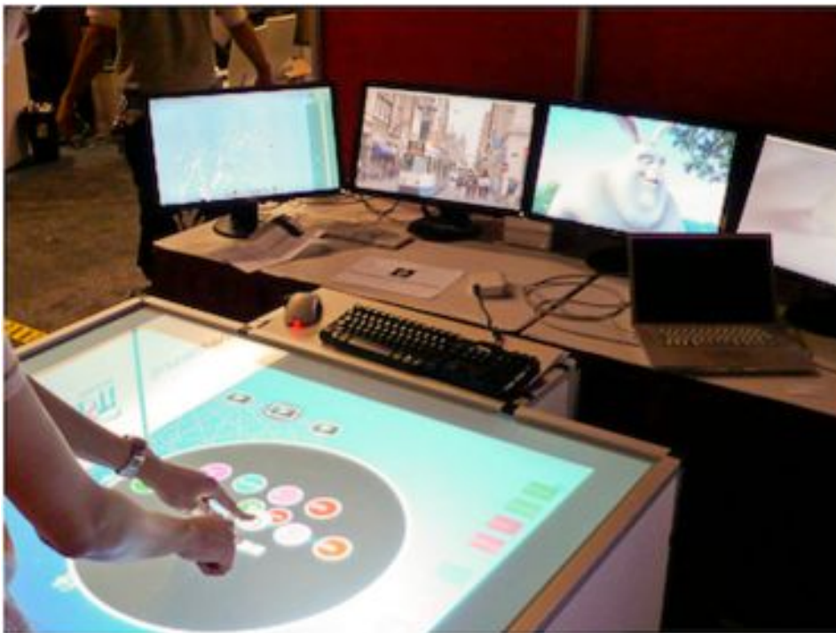
Figure 9. Modifying the sampling rate of a flow. The extreme left shows the manipulated stream, and the screen immediately to its right shows an unmodified stream that is also part of the same multicast tree.
