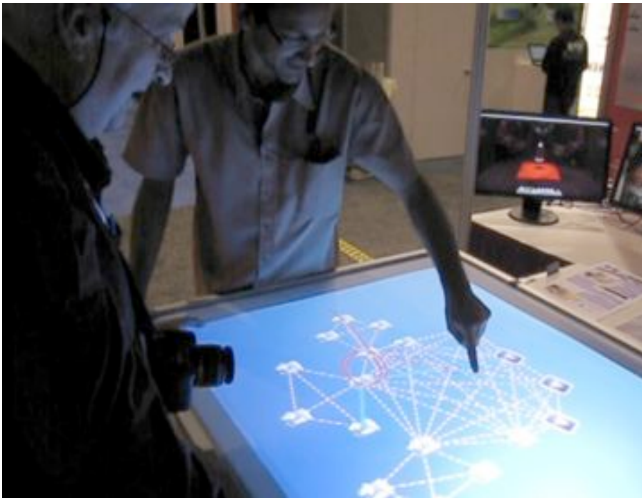
Figure 6. Creating a loop. Unicast paths can be routed any way a user likes, whether it contains one or more loops or crossings. The compiler will detect and generate the correct expressions.
