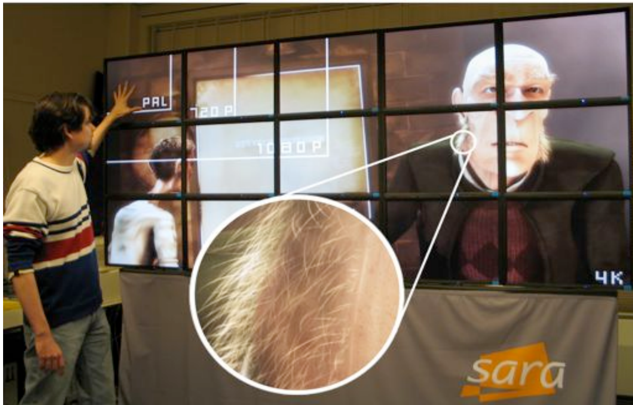
The slide above shows the visualization of cinematic SHD content (3840 by 2160 pixels) on a tiled display setup at the supercomputing center in Amsterdam.
